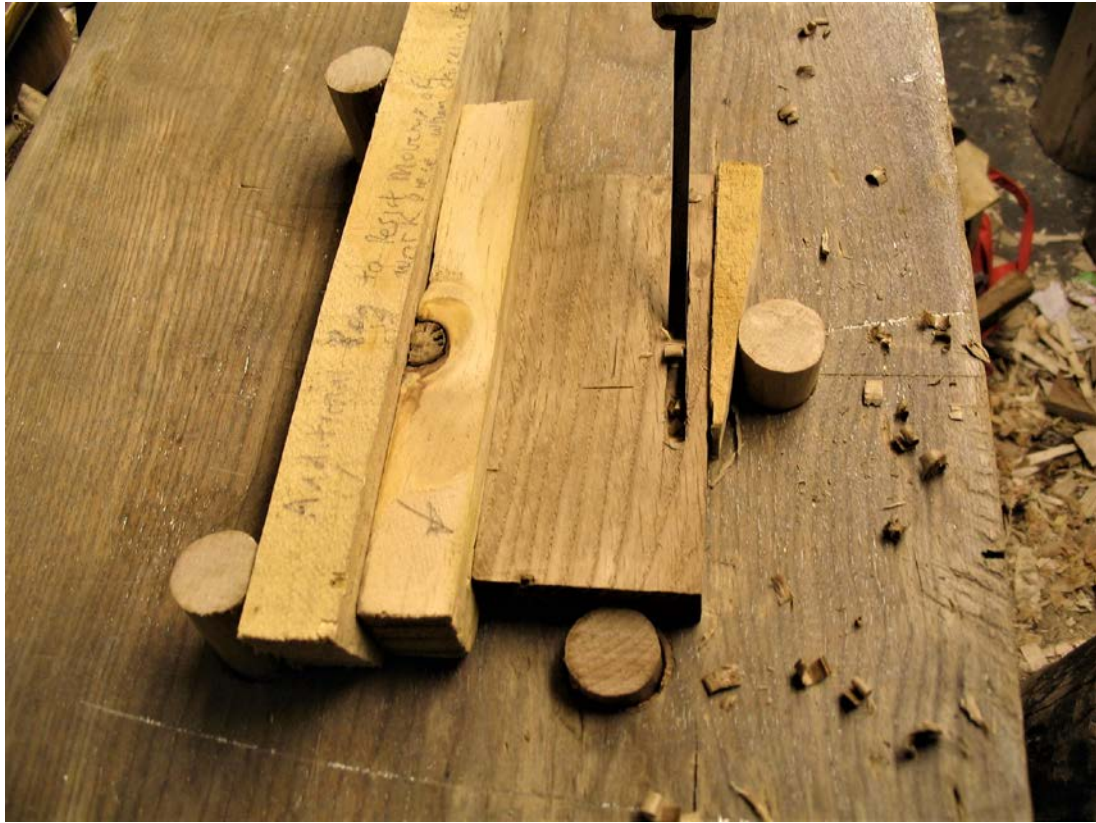
Fig. 7. The pegs and wedges in action, chiselling work on top of the bench
